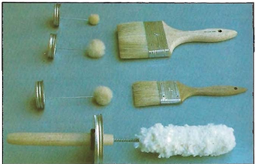
Daubers, brushes and a mop illustrate the various sizes and styles of cement applicators.
